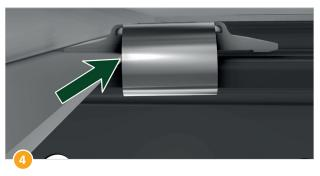
Clamping clasp must rest against module frame.
