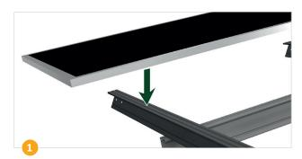
Place the solar module onto the Z-purlin.
