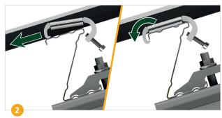
Push clamp over Z-purlin. **Attention:** do not damage back foil!
