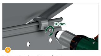
Tighten M6 bolt to 10 Nm +/- 0.5.
